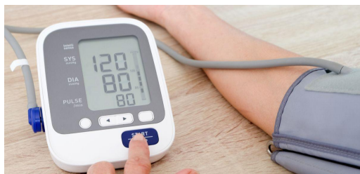
Fig. 2 A digital blood pressure monitor being used to measure someone's blood pressure. The monitor displays systolic and diastolic pressure readings, along with pulse rate. The image highlights the arm cuff connected to the monitor, which is wrapped around the person's upper arm. Kario & Tomitani (2021) advanced blood pressure monitoring devices. Retrieved from https://doi.org/10.1038/s41440-021-00671-3
